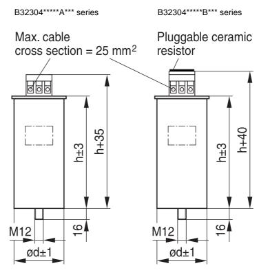
Torque = 10 Nm, Toothed washer J12 DIN 6797, Hex nut BM 12 DIN 439
