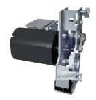
The closing spring is charged by an electric motor. When the breaker is closed, the spring is charged automatically (ON-charge method.) The closing coil (CC) is required to remotely close, and the shunt trip device is required to remotely open the breaker.
