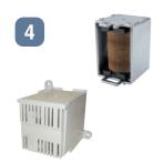
This is the device that automatically trips the breaker when the circuit voltage drops below the nominal voltage, and comprises UVT coil and UVT controller. There are 3 kinds of tripping time, INST, 0.5s and 3.0s. A trip terminal for forced OFF function is included as standard equipment.
