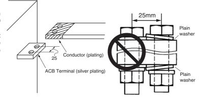
Since fault current flowing through the conductors cause large electromagnetic forces, the conductors should be secured firmly, using the values in the below table as a reference. Max. distance between fixing support and ACB bus bar should be less than 200mm.
