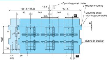
The mounting angle should be prepared by the customer.
