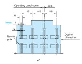
Note) Spacers are not required when fastening connecting conductors (T10). The necessary contact area can be obtained with ACB terminal bent by tightening the screw.
