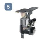
OCR alarm (AL) is provided as standard if ETR is equipped. OCR alarm (AL) is the contact (1a) of short-time operation (30ms), being output when the breaker is tripped by the electronic trip relay. Two types of automatic reset type (standard) and manual reset type (optional) are available. When ordering, specify either automatic reset or Manual reset.
