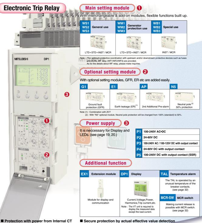
The Over current protection and Ground fault protection can work with power from Internal CT, even if the control power source is off. For the Trip indicator LED
